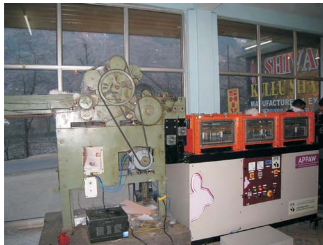
Figure B.1.3.1 Atmospheric pressure plasma processing system for Angora wool installed at CWDB, Kullu, Himanchal Pradesh, India.
