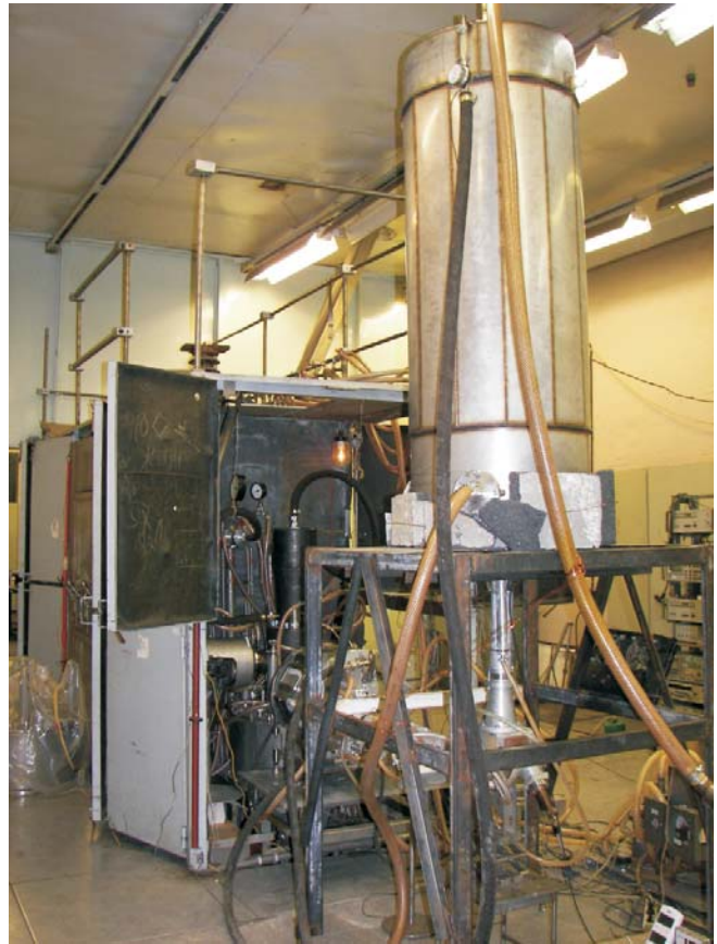
Figure A.1.2.4.5 High power Gyrotron test with Calorimetric dummy load
