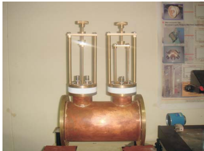
Figure A.1.2.4.1 Directional coupler for high power measurement
